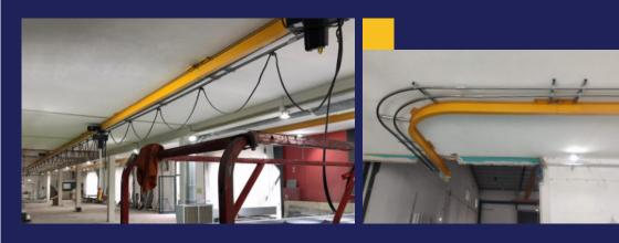
The ideal solution for moving light loads. The EUROSYSTEM can take the form of a monorail, single-girder cranes or even double girder cranes.
