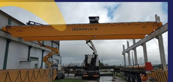
Used for indoor and outdoor services, this equipment is manufactured in the most diverse capacities. They are a viable solution when the span is too big, or the building cannot support lifting loads via overhead cranes. At the same time, it also allows the movement of loads under cranes, thus increasing their roductivity.
